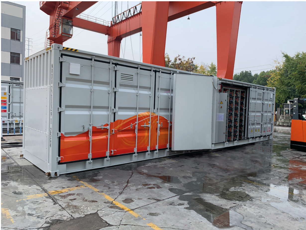
BESS Factory Audit (Source: Sinovoltaics)
