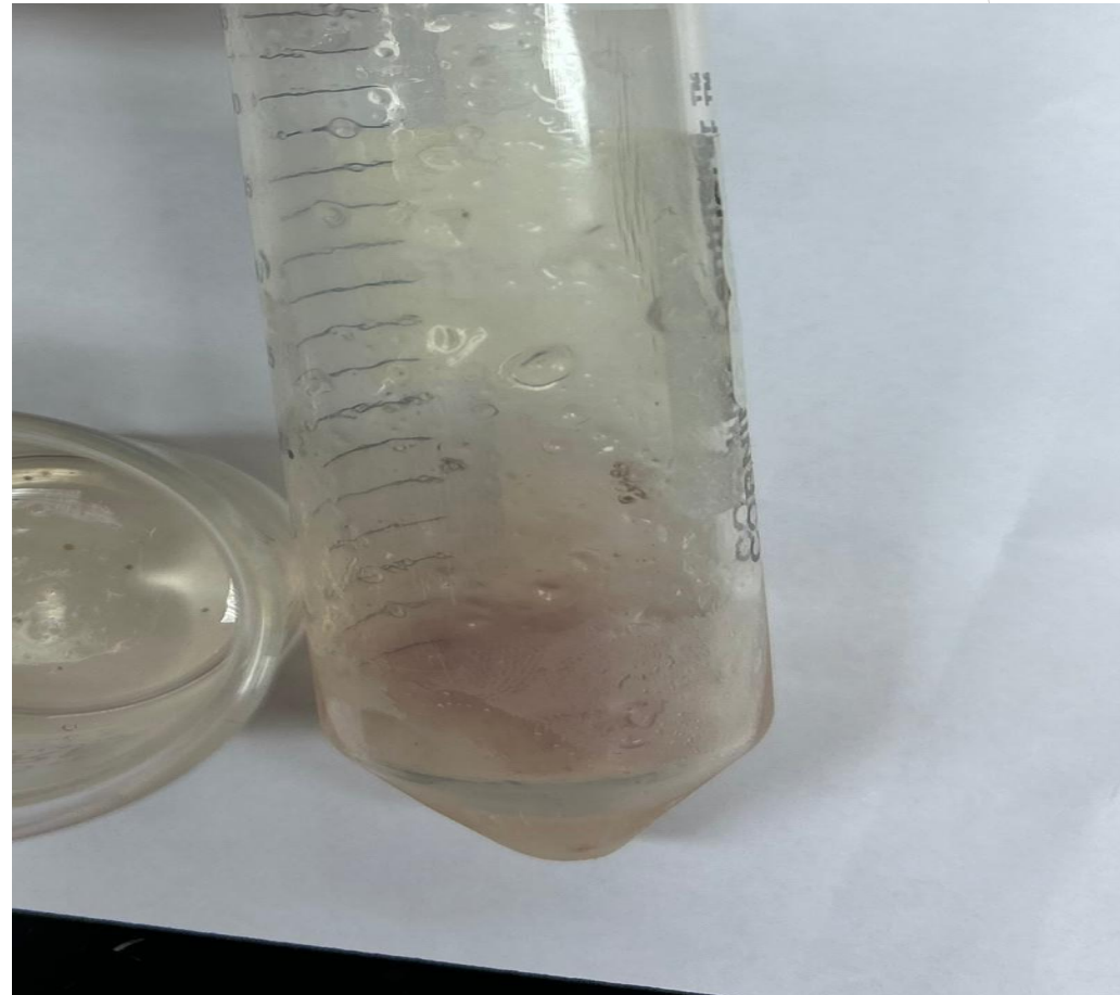
Coagulation due to the extraction at 40 degrees Celsius
