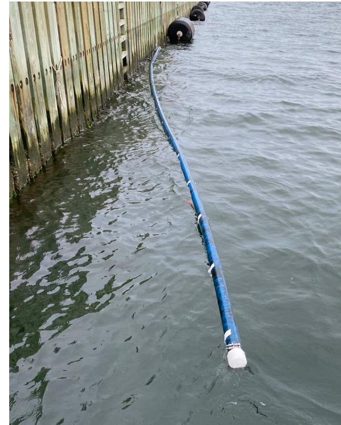
An anchorless, inflatable-hose set line
