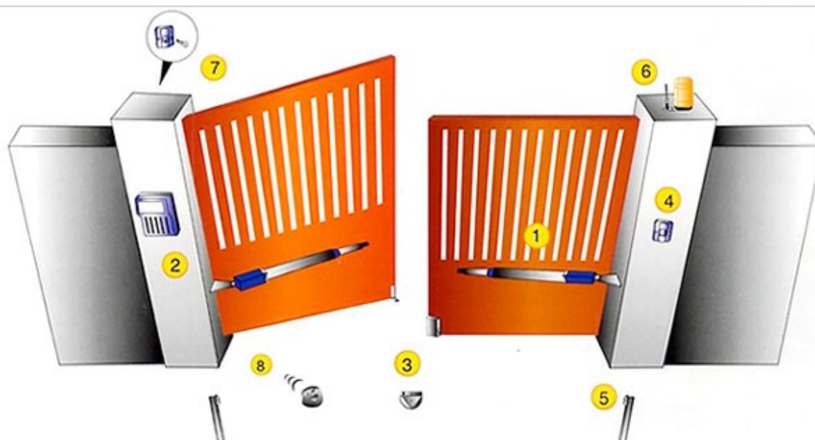
1.GATE OPERATORS 2.CONTROL BOX 3.ELECTRIC LATCH AND STOPPER 4.PUSH BUTTON 5.THROUGH BEAM TYPE INFRA-RED PHOTO SENSOR 6.FLASHING LIGHT/ANTENNA 7.KEY SELECTOR 8.TRANSMITTER
