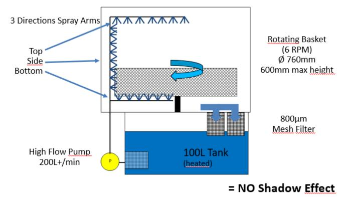
A typical cleaning cycle take about 10 minutes. A complete cycle including Rinsing and Drying can be completed within 30 minutes, depending on the application and contamination
