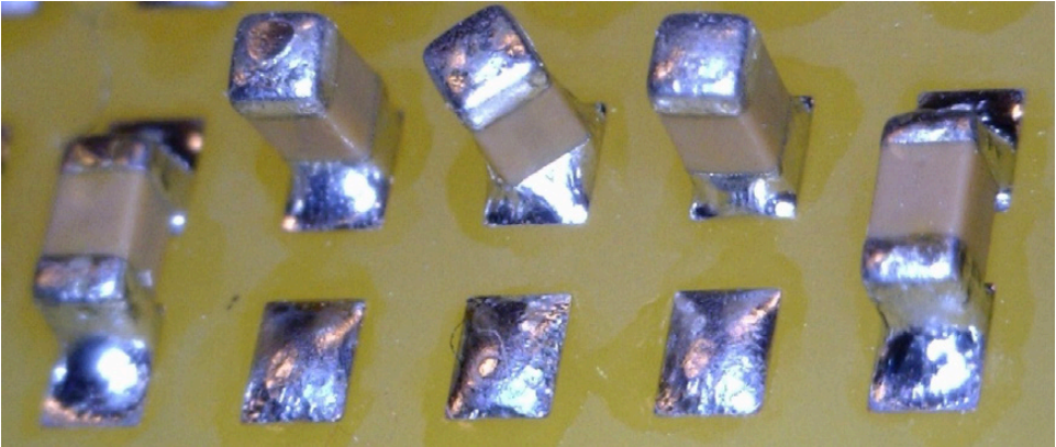
Figure 4.1: Tombstoned capacitor components.
