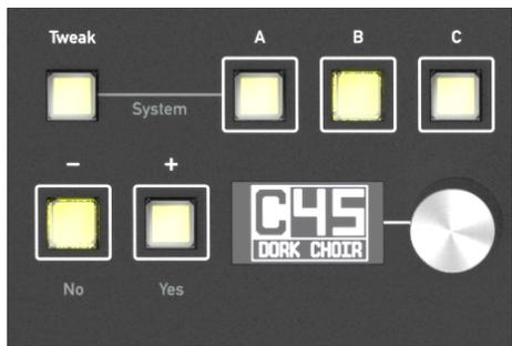
Five tweak slots are available, each consisting of a source, an amount and a destination. Once the source is selected and not set to *off*, the second column shows a numeric amount constant from 0 to 127. Depending on the selected source, the destination is affected in different ways. The fifth tweak slot is special because the amount itself can be tweaked. Sources can be any of these:
