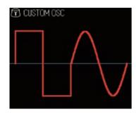
OSC1 and OSC2 waveforms are blended cyclically over the PERIOD and output. For example, if PERIOD is 1.0, OSC1 is Sine and OSC2 is Square, the output waveform will change from sine to square and back to sine each period.
