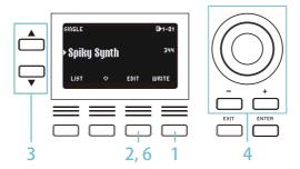
2 Press the function button that's below EDIT in the display. The parameter is shown in the display.
