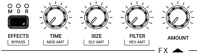
UNO Synth PRO X is equipped with 3 slots of digital effects, which are MODulation, DELAY and REVERB. There is also an Analog DRIVE in the global section.
