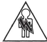
The lightning flash with the arrowhead symbol superimposed across a graphical representation of a person, within an equilateral triangle, is intended to alert the user to the presence of uninsulated "dangerous voltage" within the product's enclosure; that may be of sufficient magnitude to constitute a risk of electric shock.
