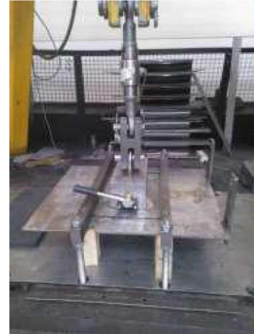
Figure 3: test set-up for the determination of the break-away force
