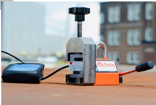
The perpendicular force measurement Pull force testing set
