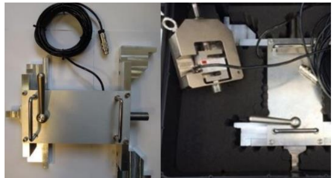
Shear force testing set
