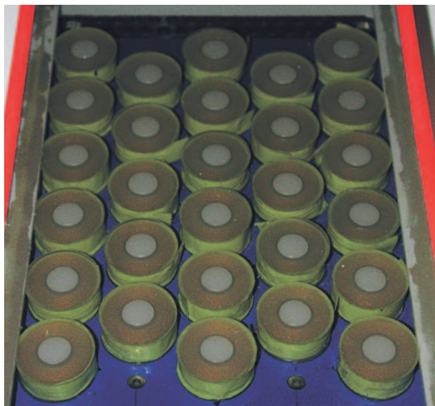
Fig. 4 Coilbed. Close up of the structure of the coils used for stimulation.
