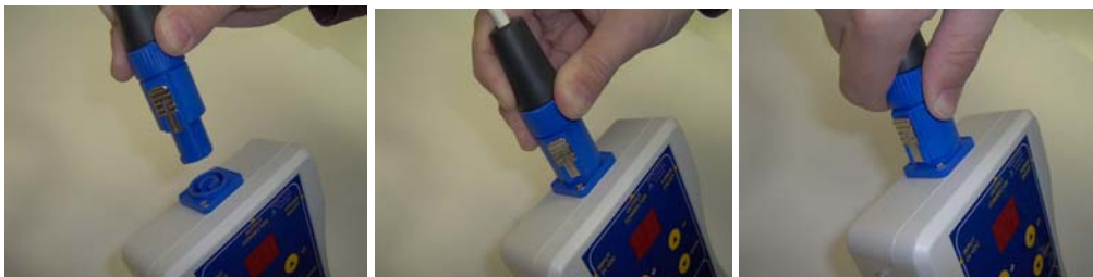
Figure #2: Connecting Output Connector to Handheld Controller
