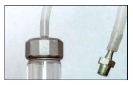
Designed to vent air from the Column's top back to the equipment headspace, creating a closed loop and leveraging any installed desiccant breather. **Included:** Stainless steel barbed fittings at each end (1" NPT female, 1/8" NPT male), 6' length of 1/4" ID LLDPE tubing.
