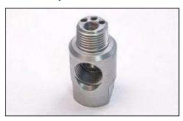
Splits a 1/2" NPT fill port into two independent ports for filling and breathing. Enables simultaneous filling and breathing without contamination. The 1/8" port can also connect to the Column Vent Tube Kit. **Ports:** 1/2" NPT female fill port; 1/2" and 1/8" NPT female breathing ports.
