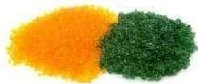
The silica gel turns from yellow to green
