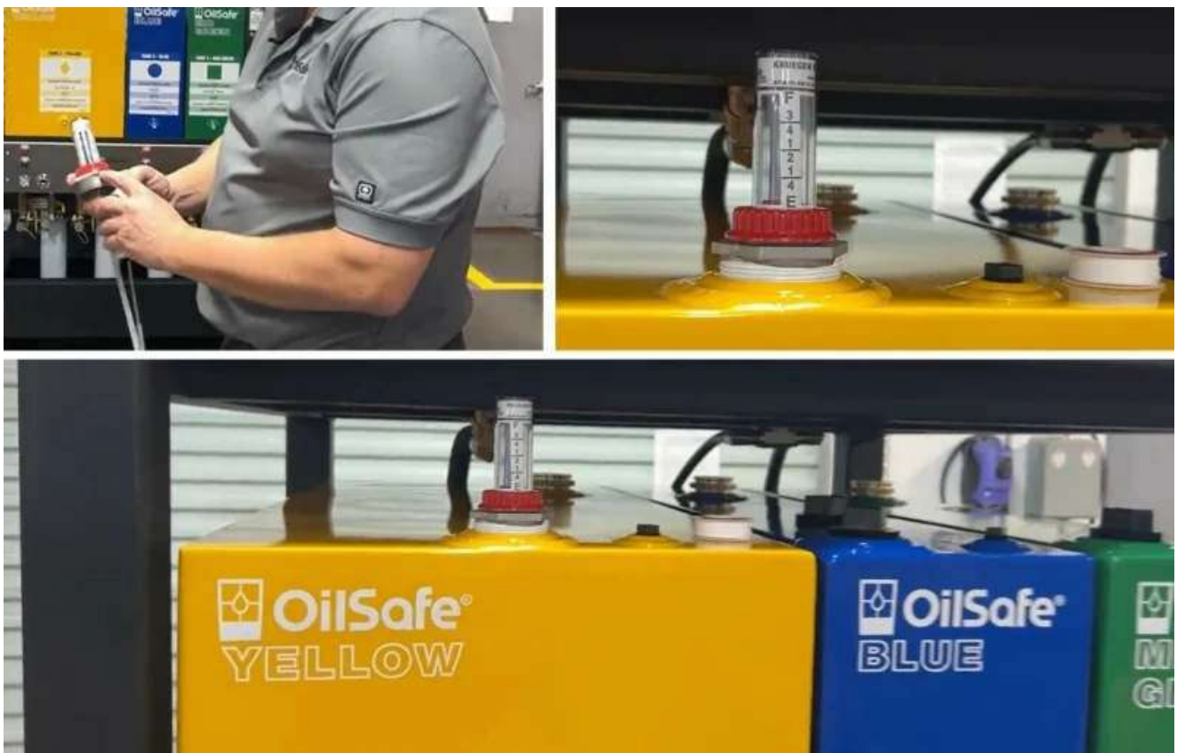
Installing the float level gauge
