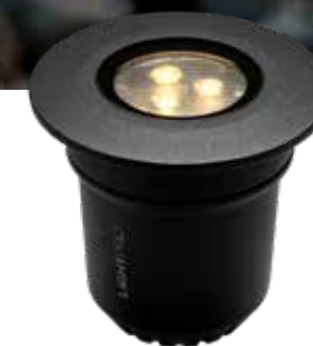
Nomia [207U] Aluminium - zwart LED 3W 3.000K - 313lm 86 x 90 mm (HxØ) Boorgat 70 mm
