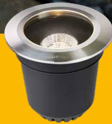
Atik R2 [187U] RVS 316 LED 9W 3.000K - 750lm 115 x 120 mm (HxØ) Boorgat 100 mm
