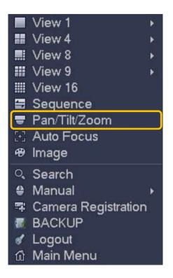
Please note the command name is grey if the device does not support this function. The PTZ operation is only valid in single window mode.
