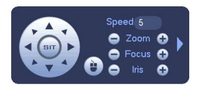
In the middle of the eight direction arrows, there is a 3D intelligent positioning key.
