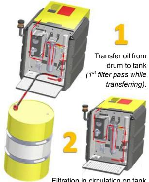
Filtration in circulation on tank (Inline circulation filtration; ideal 7-10x tank contents).
