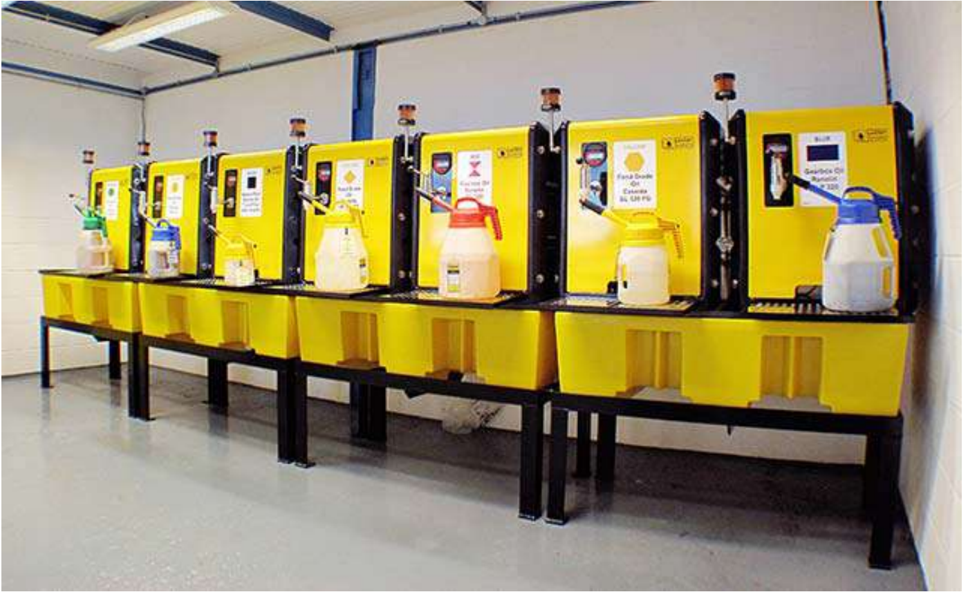
Figure 1: Lustor is a modular plug & play system. User selects the number of units, tank sizes and components based on lubricant data and will be supplied with the turnkey modules.
