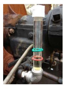
Oil Level Indicator shows an accurate level of oil inside the reservoir.
