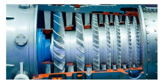
Energy reliability is essential in the world today, so scheduling turbine maintenance can improve the bottom line of any energy generating unit. Oil drains for power-generating turbines are especially expensive because they require other energy producers to cover the gap in the grid, so it's critical to extend drains intervals safely and catch maintenance problems early. Fluid analysis can determine if:
