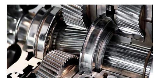
Mobile power transmissions, including differentials, final drives and planetaries are susceptible to dirt and water contamination due to their location on equipment, especially in the off-highway and mining conditions. Plus, the hydraulic qualities of automatic transmissions make them even more sensitive to dirt and water.
