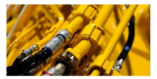
Hydraulic systems operate under extremely close tolerances and high pressure, making them susceptible to small amounts of contamination. Keeping the environment clean in industrial settings can reduce the risk of contamination, but off-highway and mining equipment expose their hydraulic systems to large amounts of dust and water.
