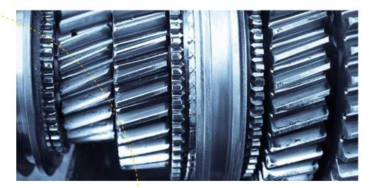
Industrial gearboxes are usually located in cleaner environments than mobile equipment. While mining, off-highway and transportation equipment is more susceptible to water and dirt contamination, vibration due to misalignment and fluid properties is a more common cause of abnormal equipment wear in industrial settings.
