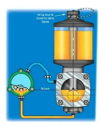
By equalizing the pressure between the oiler and the equipment the level is more accurately maintained, creating a closed-loop system.
