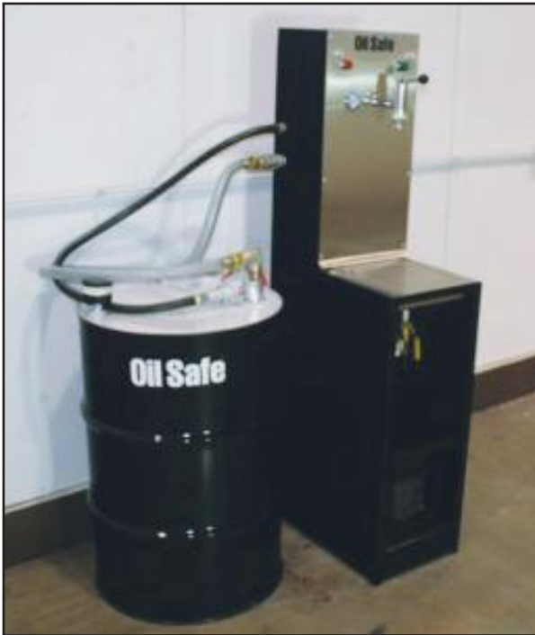
FIGURE 3: Overview of Barrel Pump Connected to Drum
