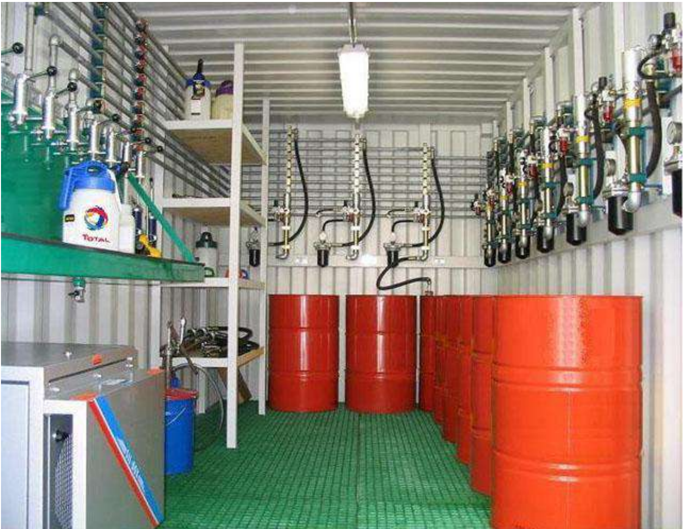
An example of a cleanliness-control center.
