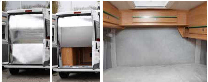
① One-piece rear door insulation
