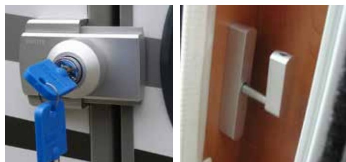
UniversalLock for body doors External locking w/ key, locking & unlocking from inside via rotary lever. Mounting possible on all motorhomes & caravans. For mounting the rotary lever, there must be a distance of min. 16 mm inside next to door. Dim.: L250 x B140 x D50 mm, weight: app. 1 kg. Scope of delivery: 1x lock with mounting material & 2 keys.
