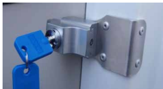
Fiat Ducato 2006-2021 For panel vans & motorhomes, installation on inside of cab doors. Left and right keyed alike. Dim.: L180 x W165 x D45 mm, weight: app. 0.9 kg. Scope of delivery: 2x lock with mounting hardware & 3 keys.
