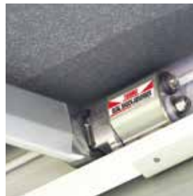
Dual-shock absorbers on support arms absorb wind movements, e.g., and thus protect awning & vehicle.
