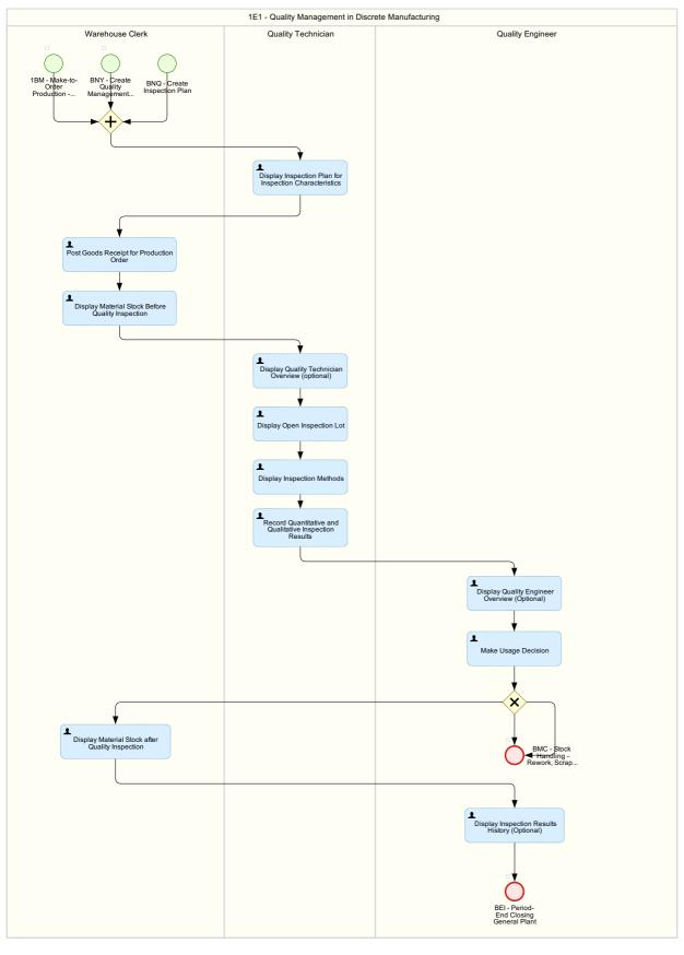
Within Production Process - Make-to-Stock Production of a Batch Managed Material
