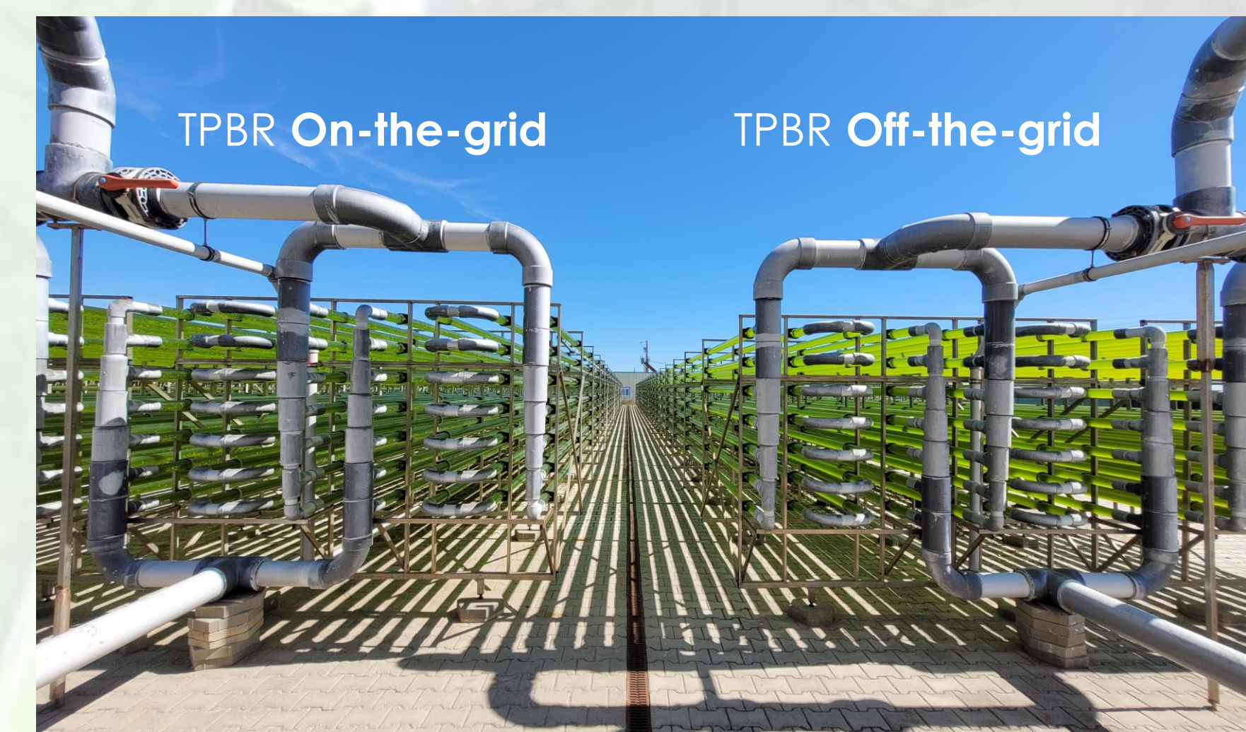
Figure 2: Systems used for the cultivation of N. oceanica . Right: 19 m 3 TPBR 4 off-the-grid; left: 19 m 3 TPBR 3 on-the-grid (Trial 1). On the on-the-grid mode, pumps work at constant speed using grid energy (normal regime). On the off-the-grid mode, pumps are stopped during the night and start increasing their speed after sunrise. Then, they work at normal speed when enough irradiance is available, but slow down when the photovoltaic production reduces (e.g., due to weather conditions), turning off again before sunset.
